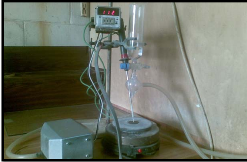
Figure (2.7) The air atomizer set up system.
